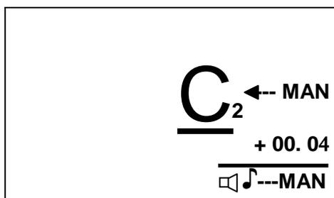
When switching from AUDIO tuner mode to VISUAL (strobe) mode, the strobe bands are once again made visible and the note selection is forced to AUTO.
