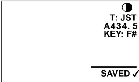
The VS-1 tuner would now power-on with these MENU item values until a new SAVE procedure is completed. The last entered tuning mode will resume when one of the MENU buttons is pressed to create a new “current MENU item” and exit SAVE mode.
