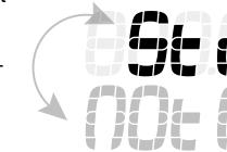
**NOTE:** When "Str" is selected, your tuner will not function as a chromatic tuner. Instead, all input signal is either sharp or flat of the exact pitch to which the displayed string number should be tuned.
