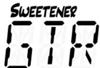
Click either the Up ( ▲ ) or Down ( ▼ ) Menu button until the 3-letter preset name flashes. Use the Plus ( + ) or Minus ( - ) Value button to select one of over 130 built-in presets. Press either Menu button to exit or allow the active, flashing parameter to time-out. To quickly set your selected preset back to the default (EQU), click either the Up ( ▲ ) or Down ( ▼ ) Menu button until the 3-letter preset name flashes. Then, click the Menu Up ( ▲ ) and Value Plus ( + ) buttons together.
