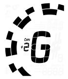
Click either the up or down Menu button until the Drop / Capo Transposition value flashes. Use the plus or minus Value button to select a value from -6 to +5. To quickly set your Drop / Capo Transposition back to the default value of 0, click either the up or down Menu button until the Drop / Capo Transposition value flashes. Then, press the Menu up and Value plus buttons together.
