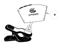
The SC-1 runs on one CR2032 coin-cell battery. To install, turn the tuner around so that its rear is facing you, remove the battery cradle from the right edge, place the battery in the cradle so that the side of the battery marked + is facing up. Slide the loaded cradle back into the tuner. A battery icon will appear when the battery is nearing depletion.
