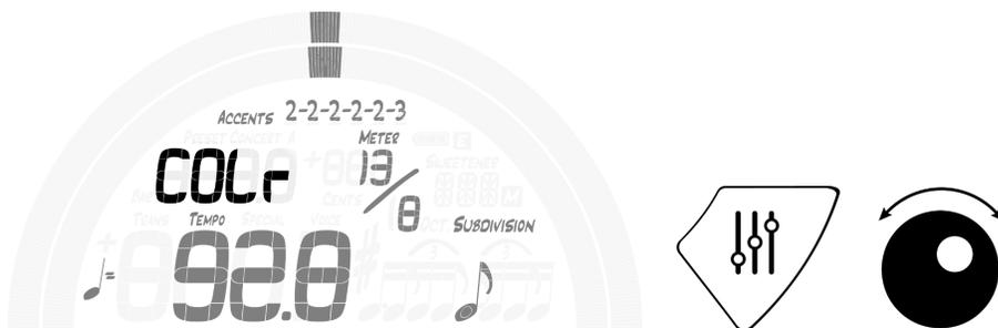
Press the parameter button until the characters COLR ( COLr ) appear and flash. Use the Value Wheel to view and select 1 of 10 predefined colors. The Preset Display Color can be useful for grouping similar presets or quickly identifying Presets and Tempo Maps when the Preset Number may be harder to see. These individually assigned Preset Display Colors are independent of and not affected by the Global Color for tuner presets set in the Settings Screen.
