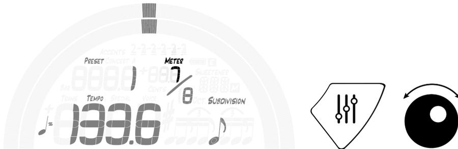
The Meter, or Time Signature, is displayed at the upper right of the metronome screen and is written like a fraction. Beats Per Measure is the numerator ( top number ) of this fraction and specifies the number of beats contained in 1 bar. Press the Parameter Button until the numerator of the Time Signature flashes and use the Value Wheel to adjust from 1 - 19 Beats Per Measure. Changing Beats Per Measure will clear any set Accent Pattern, as available Accent Patterns depend on Beats Per Measure.
