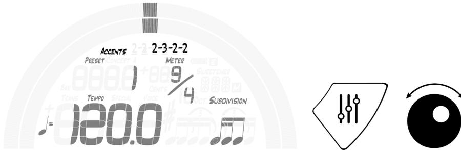
By default, the StrobePLUS HDC metronome will play the downbeat, or ‘One’ count, of every bar using a slightly higher pitch and volume than the remainder of beats. Accent Patterns help to divide and count Meters with extended Beats Per Measure settings. For example, a Meter such as 9 / x is rarely counted as One, Two, Three .... Nine. An Accent Pattern setting of 2 - 2 - 3 - 2 allows the Meter to be felt as:
