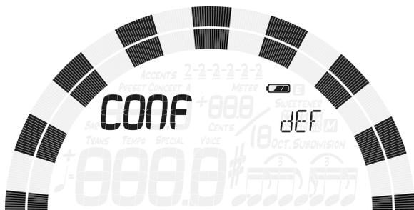
A Configuration is a collection of all the user-adjustable parameters that affect how your StrobePLUS HDC functions. This collection includes the parameters accessible in your settings screen as well as all of your Presets. Out of the box, there is only one selectable configuration named 'dEF' ( Default ). You can add an additional configuration via the use of Peterson
