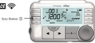
At this point, any BodyBeat Sync within range is able to join your group. Pressing and holding the ③ Sync Button subsequently ( on the Master unit ) will switch in and out of Open Registration mode allowing new members to join, or closing your group so no further members can join. Pressing and holding the ④ Sync Mode Button will break the group and return to Solo Mode. Any members who are a part of the group will be "un-syncd".
