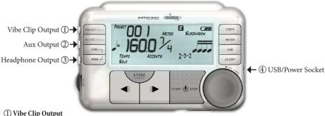
Plug the Vibe Clip into this socket and attach the Vibe Clip to your belt to feel the beat. When connected, the Vibe Clip will shut off the internal speaker.
