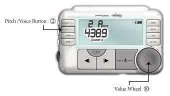
*Note:* Pressing the (**i**) Start/Stop button at any time while in Tuning Mode will revert back to Metronome Mode and begin playing the current Metronome settings. Also, pressing any button related to the metronome function will revert to Metronome mode.
