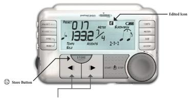
Navigate through your stored Presets by using the Next and Previous buttons. Holding either button will gradually increase the rate of selection in the respective direction.
