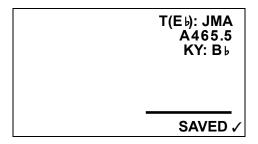
The V-SAM unit would now power-up with these MENU ITEM values until a new SAVE procedure is completed. The last entered V-SAM mode will resume when one of the MENU buttons is pressed to activate a new "current MENU ITEM" and exit the SAVE screen. Saving MENU ITEM values under the Strobe, Audio Tone, Metronome, and Light modes works in identical fashion.
