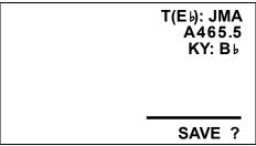
At this point, the current values of the savable menu items are displayed so that you can review the values you will be saving. Pressing either MENU button at this point will cause a new MENU ITEM to become current and no saving operation will have occurred. By either turning the VALUE knob or pressing the CHOOSE button once, however, a "confirmation" screen will appear:
