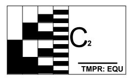
The 3-letter acronym after this indicates the current setting for temperament. **NOTE:** if not "EQU" (the default setting), the non-default status will also appear at the upper right portion of the display as described in the "**RUN Screens In More Depth—Status Displays**" section below.
