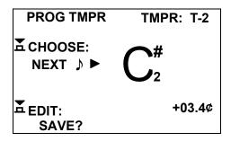
Under the **EDIT** SAVE screen, a first push of the CHOOSE button calls a SURE ?? confirmation screen. A second push of the CHOOSE button will actually save—after a short delay—all the scale note presets entered (or left unchanged) for the currently selected temperament file. The SAVE function can be aborted by pushing the EDIT button or dialing the VALUE knob one position instead of pushing CHOOSE again during the SURE ?? confirmation screen.
