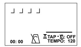
Starting and stopping the metronome as well as tapping in a tempo are all accomplished with the CHOOSE button at a single MENU ITEM selection: the screen which first appears when entering Metronome mode. This is indicated at the screen line with the  $\Xi$  (CHOOSE button symbol) shown above.
