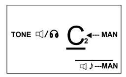
• After a brief delay, a tone will be audible from the internal speaker at whatever scale note and offsets were last registered as indicated on the screen. The speaker will be cut off when any 1/4" plug—usually a stereo headphone or mono line to an amp or PA—is plugged into the ack.
