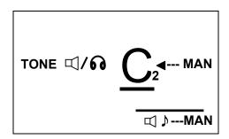
When switching from Audio Tone mode to Strobe (visual) mode, the strobe bands are once again made visible and the note selection is forced to AUTO but can be changed to MANual if desired.
