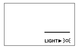
Rotating the VALUE knob or pushing the CHOOSE button will alter the backlight between  $\gt O \le$  (on) and ① (dim). (The "dim" setting cuts battery drain by  $\sim 40\%$ .)
