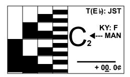
If the A4 menu item is then changed to a non-default value (even if it is not saved) by pressing one of the MENU buttons to make A4 the "current MENU ITEM" in the bottom text line and turning the VALUE rotary knob to display a value of, say, 440.5, then the non-default status of A4 will appear in its given position (second text line). These non-default status displays will remain even when a new current MENU ITEM (¢, for example) is selected:
